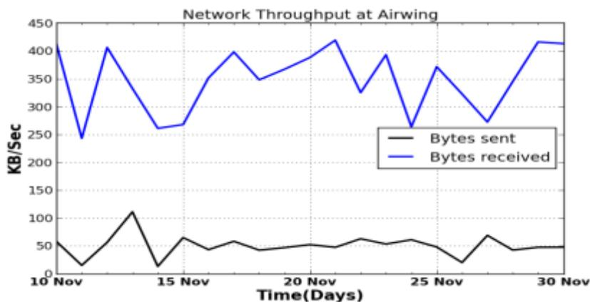
Fig. 4: Average downstream throughput at Airwing TVWS station (7.5 km from BS).
