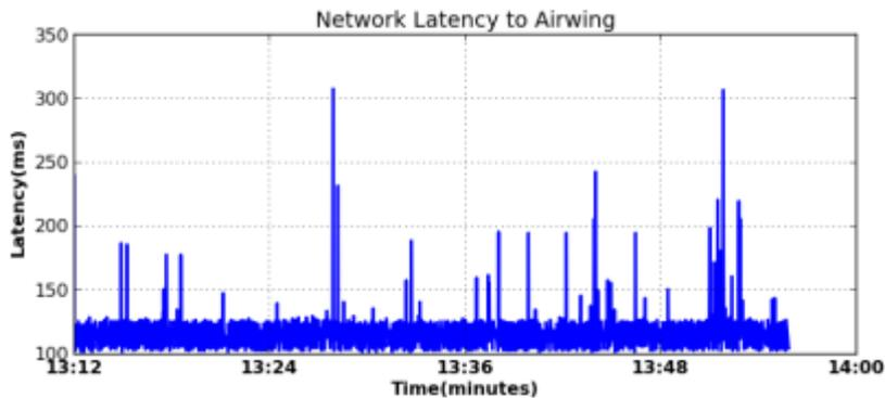
Fig. 5: One hour latency measurement at AirWing station
