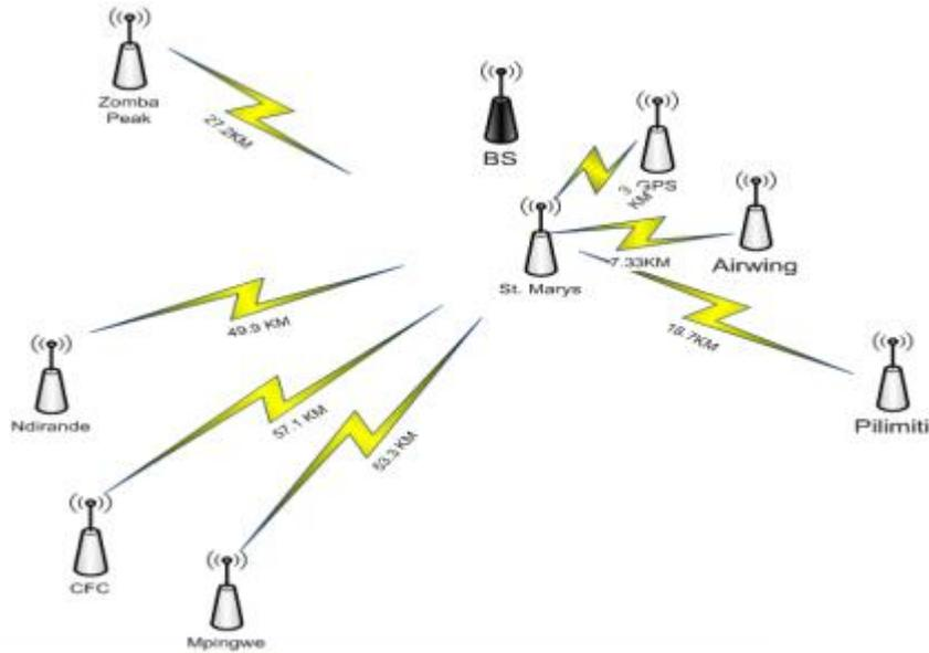
Fig. 2: UHF and TVWS network. The network covers the following districts; Zomba, Chiradzulu, Blantyre, Machinga, Mwanza and Phalombe covering a total area of 9,870 km<sup>2</sup>
