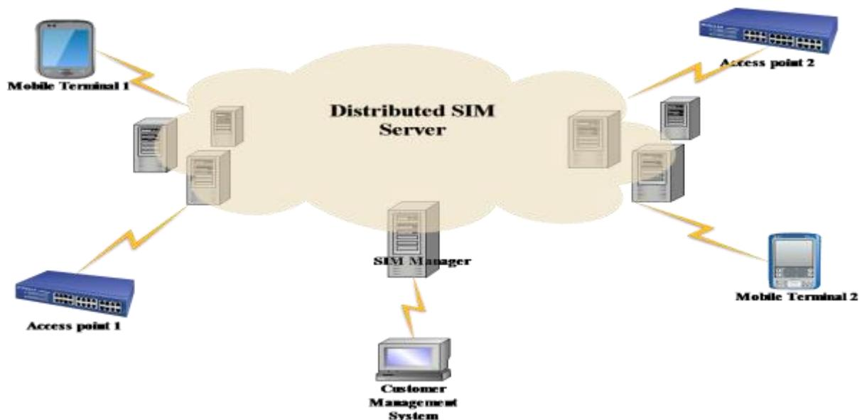
Figure 3: Implementa Virtual SIM Platform Architecture [8]
