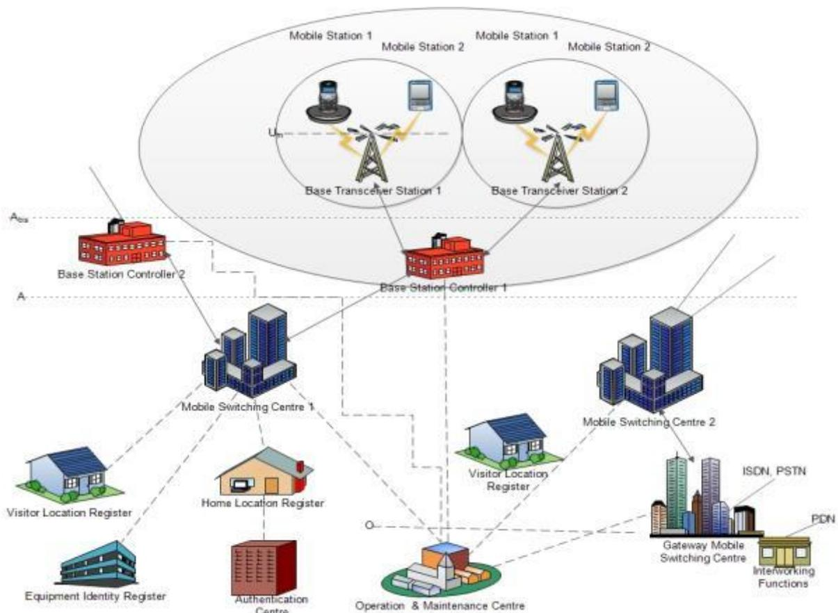
Figure 1: GSM Architecture
