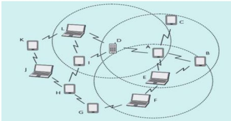
Figure 3. Routing knowledge of node A when it communicates with nodes B, F and J
