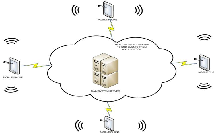
Figure 2. Proposed Mobile Ad Hoc Network diagram
