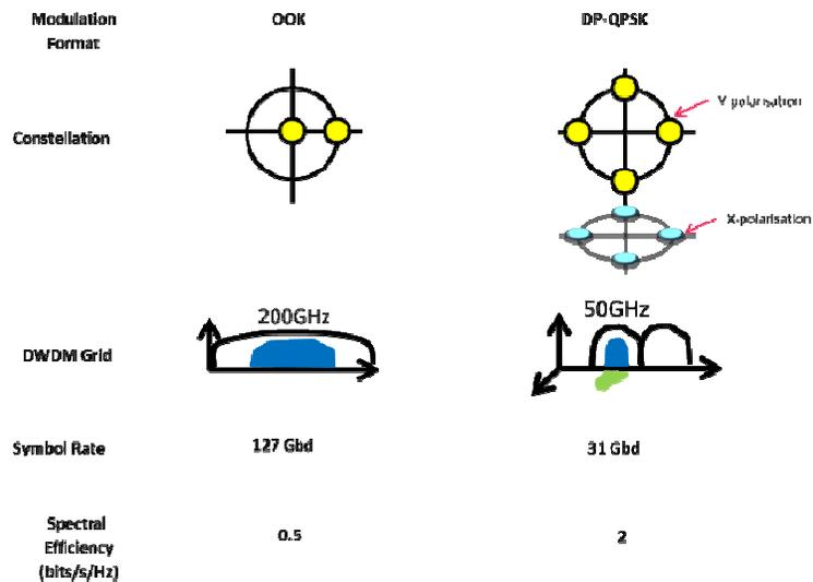
Figure 4: Comparison of modulation formats for 100 Gb/s DWDM transmission
