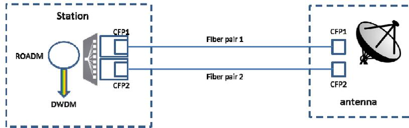
(b) 100-GbE direct-on fiber connection between antenna and station using CFP
