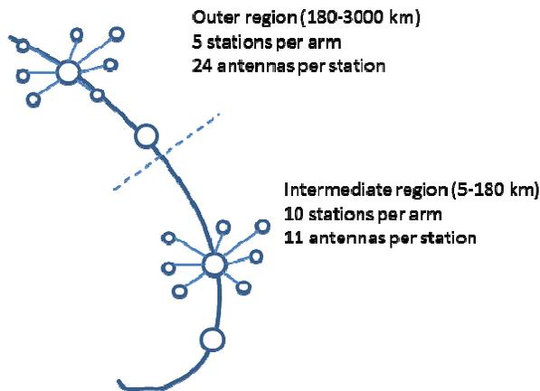
Figure 3: Potential configuration of stations and antennas in outer regions
