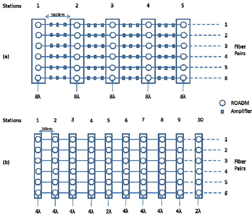
Figure 5: Potential architecture for the (a) 5 stations in the outer region and (b) 10 stations in the intermediate region of the spiral arm
