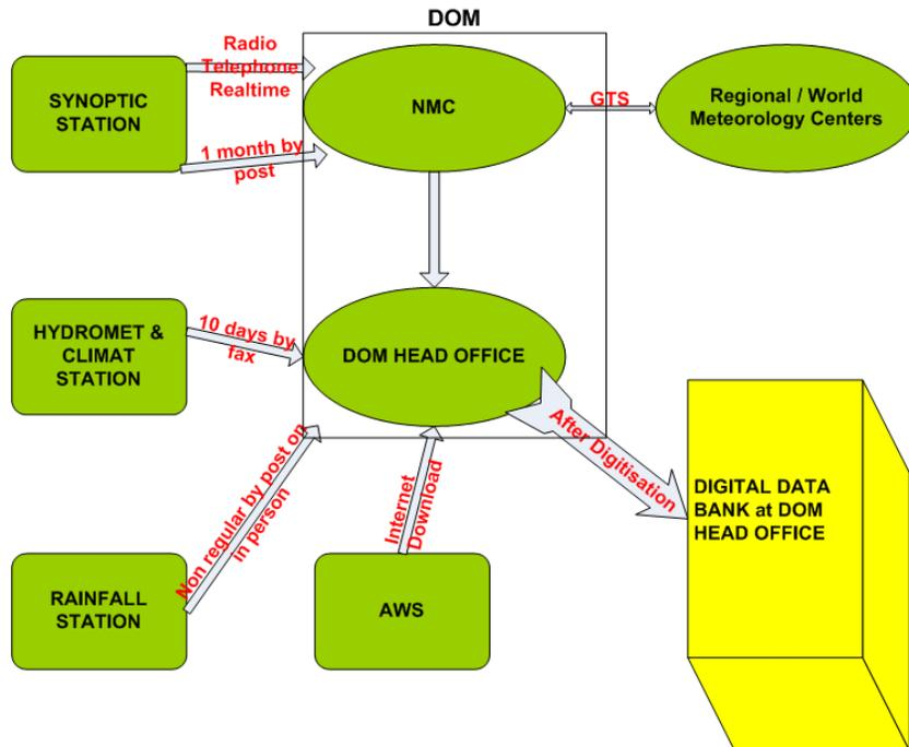
Figure 2: Data Flow from Weather stations in Uganda (source: DOM)
